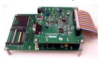
Figure 1-4. TUSB3210 Printed-Circuit Board (REV 1.1)—Top Side
